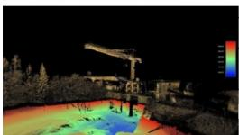
The Seabed Lidar system, equipped with a <u>Puck sensor</u>, provides complete above-water point cloud data and can operate in harsh maritime conditions. The system conducts 3D data capture of intricate measurements of inshore, nearshore and inland waterways from up to 100 metres away. It is designed to be simple to mobilize and easy to use without the need for specialized training or qualifications, delivering rapid results that can save time and money.
