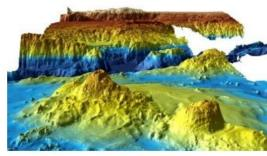
The release at the end of July 2017 of bathymetry data by Geoscience Australia has revealed seafloor maps with a resolution 15 times higher than those previously produced using satellite data. The bathymetric survey, conducted by Fugro during Phase One of the search for missing flight MH370, has provided a detailed map of the seafloor topography in the search area. The seafloor data is
