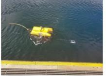
Seamor Marine's Chinook ROV is making waves in the field of undetonated explosive ordnance (UXO) detection after successfully integrating a compact magnetometer together with subsea engineers at Ocean Floor Geophysics.
