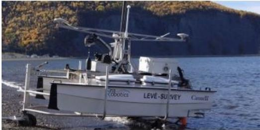
SeaRobotics recently announced the delivery of two additional 2.5m autonomous unmanned surface vehicles (USVs) to the Canadian Hydrographic Service (CHS), a part of Fisheries and Oceans Canada, bringing the fleet to four systems. These USVs, built by SeaRobotics, are complete hydrographic systems including multibeam echosounders, support sensors, cast winches, deployment carts and road trailers.
