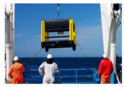
MacArtney has supplied a second <u>Triaxus</u> ROTV for use on the research vessel *RV Investigator*. This Triaxus E version features an even higher payload capacity and enables the installation of a wide range of sensors targeted to the specific needs of oceanographic research.
