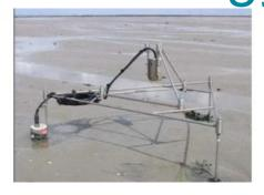
Partrac, UK, has introduced the Genesis Altimeter, a technology designed to measure small-scale changes on seabed elevation levels. The device takes high-resolution measurements of sediment erosion and deposition on the seabed, enabling users to determine the impacts of sediment movements on ecological and environmental systems.
