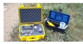
Aquatec Group has expanded the 'Sediment? Solved' range to include instrumentation to measure surface sediment stability, with the addition of Partrac's benthic flumes and Cohesive Strength Meter (CSM). The Cohesive Strength Meter is a field instrument that directly measures the surface erodibility of marine, fluvial and terrestrial sediments. It permits rapid assessment of sediment
