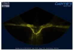
Tritech's latest product in the Gemini Multibeam range, the Gemini Narrow Beam Imager (NBI), has been used in extremely limited visibility conditions. The Gemini NBI was successfully used by Reef Subsea to monitor the trenched installation of 6-inch and 2-inch cables, while using controlled flow excavation techniques. The seabed conditions around the site varied considerably, however, even where there was high turbidity Reef was able to clearly monitor the cables using the device.
