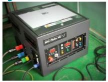
China Eastern Normal University has purchased the SIG Pulse M2 system for students who are training in marine seismic data capture and processing. They will be using sparker and boomer techniques with the same energy source SIG Pulse M2 which delivers from 100 to 2,000 joules. The sea acceptance tests (SAT) of June 2014 were performed around the Zhoushang Islands, one of the most famous China East Sea fishing locations.
