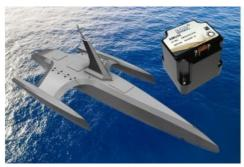
Two Silicon Sensing Systems ultra-precise AMU30 inertial measurement units (IMUs) will provide critical navigation data to the autopilot capability for the Mayflower Autonomous Ship (MAS) throughout her milestone transatlantic voyage this autumn. Setting sail this September, the 15-meter long, 5-ton MAS400 will repeat the Mayflower's original epic voyage made 400 years ago.
