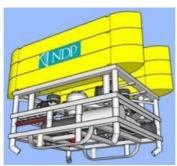
ROVLATIS joins a new generation of  Smart ROVs' and serves as a host platform for the testing and commercial spin-out of new ROV and mission support technologies within the international marine sector. Designed and developed by the Mobile & Marine Robotics Research Centre at the University of Limerick, Ireland, ROVLATIS differs from other survey class ROVs of its size in a number of key areas.
