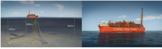
Mooring solutions supplier, SOFEC, Inc., has selected BMT and Sonardyne Inc., under their teaming agreement, to supply an innovative mooring monitoring system (MMS) for a major new deepwater development. The new system will involve monitoring of the turret mooring system on a new-build floating liquefied natural gas (FLNG) facility being built in South Korea for ENI's Coral South project offshore
