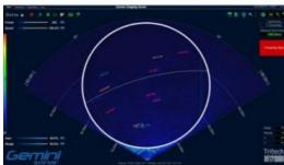
Gemini SeaTec, UK, provides an early warning of the presence of marine mammals in the vicinity of marine current turbine structures. The Gemini SeaTec system has been successfully field-tested on the Marine Current Turbine (MCT) SeaGen installation in Strangford Lough, Northern Ireland, overseen and tested by the Sea Mammal Research Unit (SMRU) Ltd.
