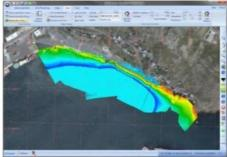
Chesapeake Technology (USA) has made further developments to its SonarWiz processing package with the addition of a real-time acquisition server for the EdgeTech 4600 and recently introduced EdgeTech 6205 interferometric bathymetry systems. SonarWiz can now capture and map real-time bathy data along with the sidescan data. It offers a simpler way to capture and visualise the data in real time.
