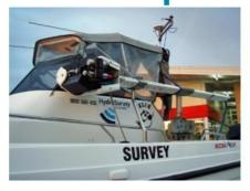
Two GeoSwath wide-swath bathymetric sonars are being used for regular hydrographic port surveys around the South Australian coast, providing bathymetry and side-scan data for use in the development and maintenance of this national infrastructure. Recent projects include the pre, progress, and post-dredge monitoring of the major shipping channels to Port Adelaide and Port Giles which were deepened to accommodate panamax vessels.
