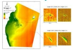
Germany-based GAF has developed and successfully demonstrated a new approach for deriving bathymetry from space. With this method, GAF can generate bathymetric maps covering large areas by simultaneously using differential spectral attenuation and stereo information from satellite imagery. The approach only requires the use of satellite stereo imagery with precise ephemeris data and is independent of ground-truth data such as echosounding or Lidar depth measurements.
