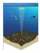
Working with NOAA's Northwest Fisheries Science Center (NWFSC), the University of Washington recently retrieved a BioSonics DTX-SUB split-beam echo-sounder after a one-month deployment in northern Admiralty Inlet, WA. The unit was detecting, categorising and counting pelagic fish, invertebrate and marine mammal species in order to determine suitable locations for tidal energy turbines.
