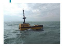
ASV Global has announced the successful deployment of one of its C-Worker 7 class of autonomous surface vessels for Subsea 7. The 7m autonomous surface vessel was used to support a pipelay operation off the coast of Egypt. Fitted with a survey suite comprising a multibeam echosounder and sidescan sonar, the C-Worker 7 carried out touchdown monitoring in support of the 'Seven Antares' pipelay vessel.
