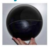
SonarBell is a passive sonar device on show during Ocean Business from 9 to 11 April 2013 in Southampton, UK. It has been developed by UK-based Subsea Asset Location Technologies (SALT) Ltd, a †spin-out' company from the Defence Science and Technology Laboratory (DSTL). The technology was first used for military applications but is now being deployed across many commercial and scientific disciplines.
