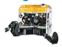
Subsea Vision has added a forth Saab Seaeye Cougar XT ROV to its fleet. The 2,000 metre-rated Cougar is to assist in unexploded ordnance (UXO) disposal. The ROV is used to locate and identify UXOs, which can include excavating the seabed to see the objects more clearly. The Cougar then lays a charge alongside the UXO, ready for remote detonation from the surface Explosive Ordnance Disposal (EOD) Officer.
