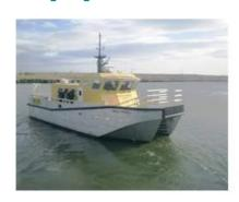
The UK boat builder Alnmaritec successfully launched a new multipurpose offshore wind farm support vessel recently. Ocean Wind 5 is a variant of the popular Wave Commander class. On deck she is fitted with a payload area both fore and aft and a substantial moon pool, and internally she has a survey station and offers comfortable accommodation for both passengers and crew.
