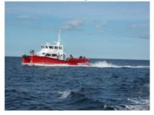
Alnmaritec has delivered Dalby Esk, the second of the new Wave Master class of wind farm support vessels, to Dalby Offshore Renewables. The new vessel has a multi-purpose capability for survey and dive support as well as wind farm service roles. She already has her first contract, working on the Outer Gabbard wind farm as a crew transfer and logistics vessel, with her prime roles being refuelling and transferring equipment around the field.
