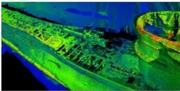
been surveyed from a Triton submersible equipped with a Sonardyne acoustically aided inertial navigation system (AAINS) and scanned by 2G Robotics' laser scanner.
