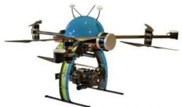
A NEXUS 800 UAS powered by HYPACK has been provided to the US southeastern geospatial solutions company SurvTech. The company will use the device to acquire upland data simultaneous with subaqueous data and make a seamless point cloud of upland and submerged data. The integration with the company's heading RTK GPS, IMU, sonar and HYPACK was experienced as straightforward.
