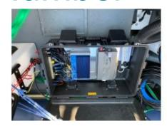
Swathe Services has announced a bespoke custom Peli-case product which has been designed to fit the surface components of an R2Sonic Multi-Beam Echo-Sounder (MBES) SIM box and Inertial Navigation System. The product is specifically designed for use in open boats such as ABP Humber's 5 metre RIB.
