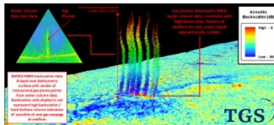
TDI-Brooks International (under contract to TGS) has completed the offshore multibeam phase offshore the Niger Delta. This survey took place in water depths of 750 to 3,500 metres and is Nigeria's first regional multi-client Multibeam and Seafloor Sampling (MB&SS) study.
