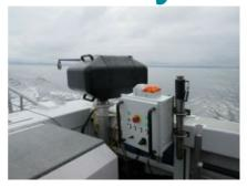
US-based Teledyne Oceanscience has announced the launch of rapidCAST, an automated sound velocity (SV) profiling system for moving vessels. With the capability to automatically cast and recover a high-quality SV probe to 500 metres at 8 knots without an operator on deck, rapidCAST offers many of the benefits previously only available from large towed profilers. Simultaneously, it offers surveyors the convenience and cost savings of a small and portable unit that is easy to mobilise.
