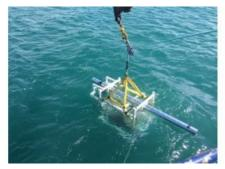
Teledyne TSS, a division of Teledyne Marine, is increasing its range of subsea pipe and cable detection and tracking products with the launch of the new smaller HydroPACT 660 pipe tracking system. The 660 has been designed to help reduce the cost of subsea pipe surveys by allowing the use of smaller classes of underwater remotely operated vehicles (ROVs). In addition, TSS is also expanding the capabilities of its larger HydroPACT 440 pipe tracking system by introducing a new 24VDC upgrade kit.
