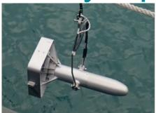
US company TerraSond, an Acteon company, has recently deployed a new Moving Vessel Profiler (MVP) to support its offshore wind farm survey operations. This is TerraSond's second MVP. AML Oceanographic's proven underway profiler was determined to be the natural solution for surveys conducted ahead of turbine foundation construction, where the importance of accurately characterizing the seabed cannot be understated.
