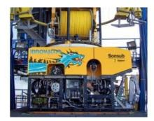
The ROV fleet of Sonsub in the UK has been augmented with the arrival of three brand new latest generation Innovator 250s. Designed and built in-house by Sonsub's own research and development team, these heavy construction class systems are capable of the highest level of activity, providing unrivalled power and control for deepwater operations, whilst retaining the now established advantages of the Innovator class.
