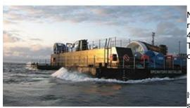
Nova Scotia Power and its technology partner, OpenHydro, have successfully completed recovery of OpenHydro's demonstration turbine from the Minas Passage. Recovery of the 400 tonne tidal turbine represents a first for OpenHydro and a first for the Bay of Fundy. The structure appears to be in excellent condition overall and, consistent with the images obtained this summer, all of the blades are missing from the centre of the unit.
