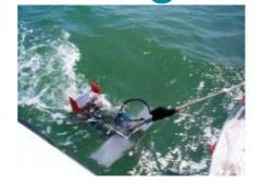
The MiniBAT Towed Coastal Monitoring Package (TCMP) is developed to addresses all coastal monitoring requirements in one easy to use system. The TCMP is based on the MiniBAT tow-body from OSIL and is fitted with YSI's 6600 Multiparameter Sonde (CTD, DO, pH, Chlorophyll, Turbidity).
