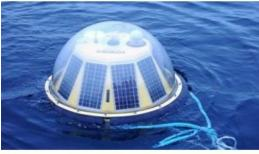
The TRIAXYS Directional Wave Buoy can be ordered with a Monitor 600 KHz Teledyne RD Instruments Acoustic Doppler Current Profiler (ADCP). The combination can provide accurate, real-time waves and currents data in virtually any water depth, without the need for divers or cables. It can also be easily mobilised for utilisation at a variety of deployment sites.
