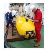
Researchers from the National Oceanographic Centre, Southampton (NOCS), recently trialled Autosub6000, a deep rated Autonomous Underwater Vehicle (AUV), to explore ocean regions approaching 6000m water depth. Autosub6000 was able to manoeuvre and avoid obstacles using Tritech's SeaKing scanning sonar. Due to the extreme conditions, a 6000m depth rated titanium SeaKing sonar was selected.
