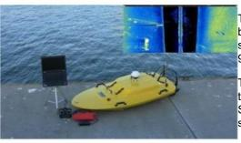
The Oceanscience Group has unveiled the first Z-Boat 1800 remotely operated survey boat with integrated sidescan sonar, from Tritech International. The new boat provides a shore operator with real-time high-definition sidescan imagery from Tritech's StarFish 990F sidescan on a portable 1.8m surface vessel.
