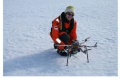
Engineers on board the Alfred Wegener Institute's research icebreaker Polarstern have programmed an unmanned autonomous vehicle (UAV), allowing it to navigate despite the deviations produced by the Earth's magnetic field near the North Pole. The researchers recently celebrated the multicopter's first successful autonomous flight and landing on an ice floe.
