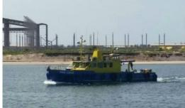
Recently, UMI SAN from Brazil took the new survey vessel St. Edwiges into service. She has a steel hull, two engines with 600HP of propulsion each, two generators and appropriate accommodation for continuous operation. The reduced sail area ensures exceptional safety and performance for hydrographic surveys in offshore areas, bringing more efficiency and quality to the work.
