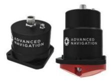
Advanced Navigation has announced the release of its Sublocus underwater navigation system. This is an underwater inertial navigation system featuring north-seeking fibre-optic gyroscopes and accelerometers with a GPS receiver and pressure depth sensor. These are fused together in Advanced Navigation's fusion algorithm to deliver positional accuracy of 0.08% of distance travelled.
