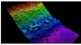
RESON is providing a SeaBat 7125 sonar system for a new breakwater mapping system GEOSUB 3DTM developed by the company MESURIS in France. It is a high-resolution 3D real-time bathymetric and topographic system designed to provide marine engineering data both above and below the water's surface, deployable either from a land or barge crane.
