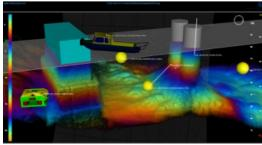
Coda Octopus, UK, has upgraded the Models+ software package which forms an optional module within its Underwater Survey Explorer platform. The capabilities of this version enable real-time live sonar data to be supplemented by static and dynamic models to allow full visualisation and management of the user's subsea â€~3D workspace'.
