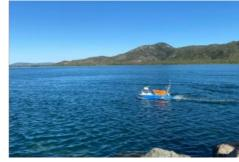
Unique Group has successfully supported the Australian Institute of Marine Science in completing a carbon-conscious bathymetric survey at Cape Ferguson by performing seabed modelling for their upcoming project, using its proprietary unmanned survey vessel, Uni-Pact.
