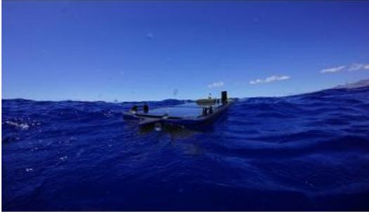
Liquid Robotics, and Boeing have for the first time used a network of persistent unmanned surface vehicles (USVs) to detect, report and track a live submarine in a naval demonstration. Four sensor hosting autonomous remote craft (SHARCs) were deployed off the coast of Northern Scotland during the British Royal Navy's Unmanned Warrior 2016 demonstration. The autonomous surface vehicles used Boeing acoustic sensors in the live anti-submarine warfare (ASW) mission.
