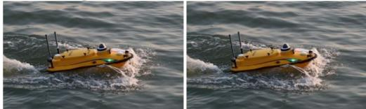
CHC Navigation (CHCNAV), a leading manufacturer of uncrewed surface vehicle (USV) technology, has introduced the Apache 3 Pro – an advanced compact hydrographic drone engineered for autonomous bathymetric surveys in shallow waters. Boasting a lightweight carbon fibre hull (IP67 rating) and a semirecessed motor, the Apache 3 Pro excels in both durability and manoeuvrability.
