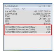
The SonarMite.dll is a singlebeam echosounder driver for the Ohmex SonarMite SBES. Having remained unchanged since it was first written years ago, it has now been updated. It appears also to give an output of roll, pitch, heave, battery condition and a current depth relative QA value in its string. Hypack has modified the drive so that it now displays the battery status in real time while in survey mode without being logged in the raw file.
