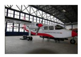
The mission equipment of the Belgian maritime surveillance aircraft OO-MMM of type Britten-Norman BN2A-21 Islander is being upgraded in the OPTIMARE hangar at the Regional Airport Bremerhaven-Luneort, Germany. The activites include the installation of the OPTIMARE's airborne maritime surveillance system MEDUSA for enhanced mission management.
