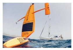
The Saildrone (SD) 1079 uncrewed vehicle has just completed a first-of-its-kind mission to remote areas of the equatorial tropical Atlantic. Sailing 11,910 nautical miles (22,057km) and spending 370 days at sea, the SD 1079 mission – part of EuroSea – was to collect CO<sub>2</sub> data to improve global carbon projections and help enable sustainable ocean resource management.
