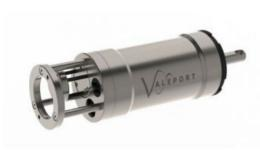
Van Oord Dredging and Marine Contractors, a leading contractor for dredging, marine engineering and offshore energy projects, has selected Valeport's SWiFT SVP for its various survey activities. The compact unit features high-accuracy sound velocity, pressure, temperature, salinity and density measurement, plus integral GPS and re-chargeable battery. Suited for coastal, harbour and inland hydrographic survey use, Van Oord is to deploy the SWiFT SVP as part of its operations worldwide.
