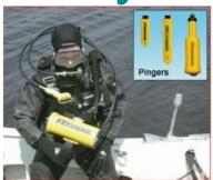
Government agencies and marine service companies are finding a variety of uses for acoustic pingers and pinger receivers. Pingers are signaling devices that can be attached to an underwater site or instrument package. Using the pinger receiver, a gun-like instrument carried by a diver, the sonar signal transmitted by the pinger can easily be detected and followed to its source.
