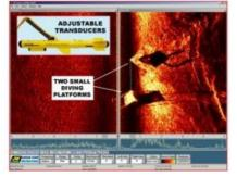
JW Fishers developed a side-scan towfish with adjustable transducers. The angle of the transducers can be changed by rotating the tail section of the towfish. This allows the sonar to scan the hull of a ship for attached contraband compartments and inspect the face of a dam, bridge, or oil platform for explosive devices.
