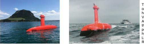
The newly created rental and services company WAMS has announced that it has added iXblue DriX Uncrewed Surface Vehicle (USV) to its pool of equipment. Available for WAMS customers in Brazil, the DriX USV will increase operational performance for shallow-water hydrographic and geophysical surveys, LBL array box-in operations and ROV/AUV tracking for deepwater projects.
